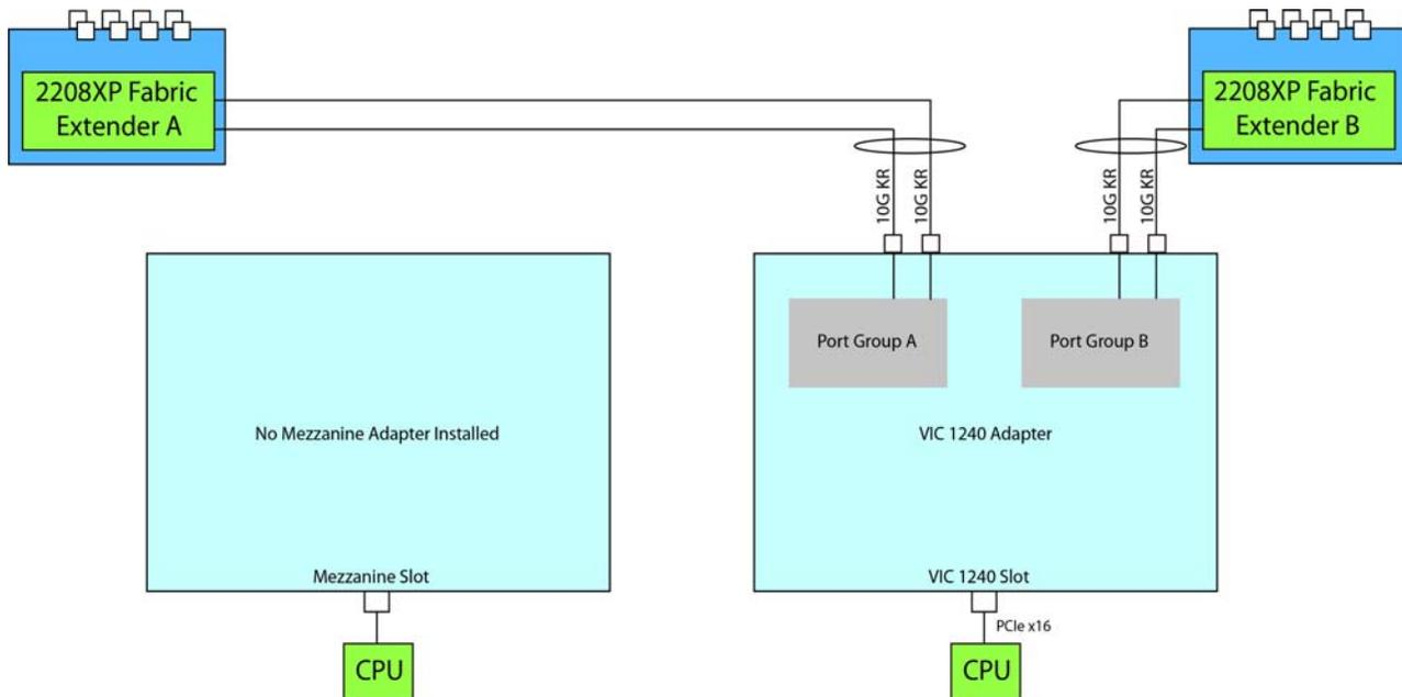
In *Figure 16*, two ports from the VIC 1240 are channeled to 2208XP Fabric Extender A and two are channeled to 2208XP Fabric Extender B. The VIC 1280 installed in the mezzanine slot also channels two ports to each of the Fabric Extenders. The result is 40 Gbps of bandwidth to each Fabric Extender.
