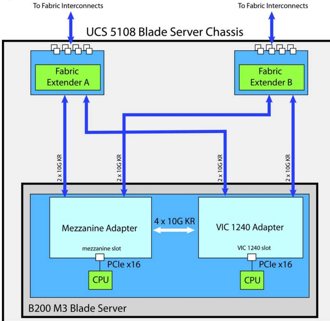
The server accommodates two types of network adapters. One is the Cisco VIC 1240 adapter. The other is a Cisco-certified I/O or flash storage mezzanine adapter. The VIC 1240 is the only adapter that can be used in the VIC 1240 slot. All other types of adapters plug into the mezzanine slot.
