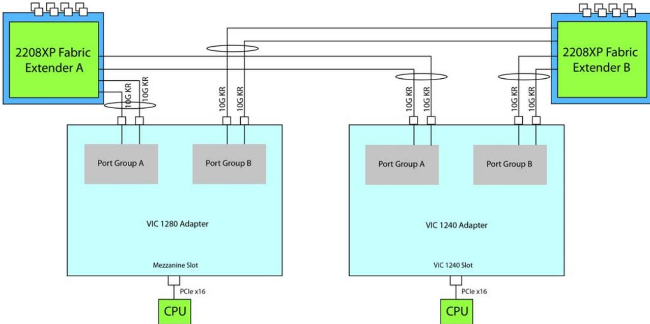
In *Figure 17*, two ports from the VIC 1240 are channeled to 2208XP Fabric Extender A and two are channeled to 2208XP Fabric Extender B. The adapter installed in the mezzanine slot also channels one port to each of the Fabric Extenders. The result is 30 Gbps of bandwidth to each Fabric Extender.
