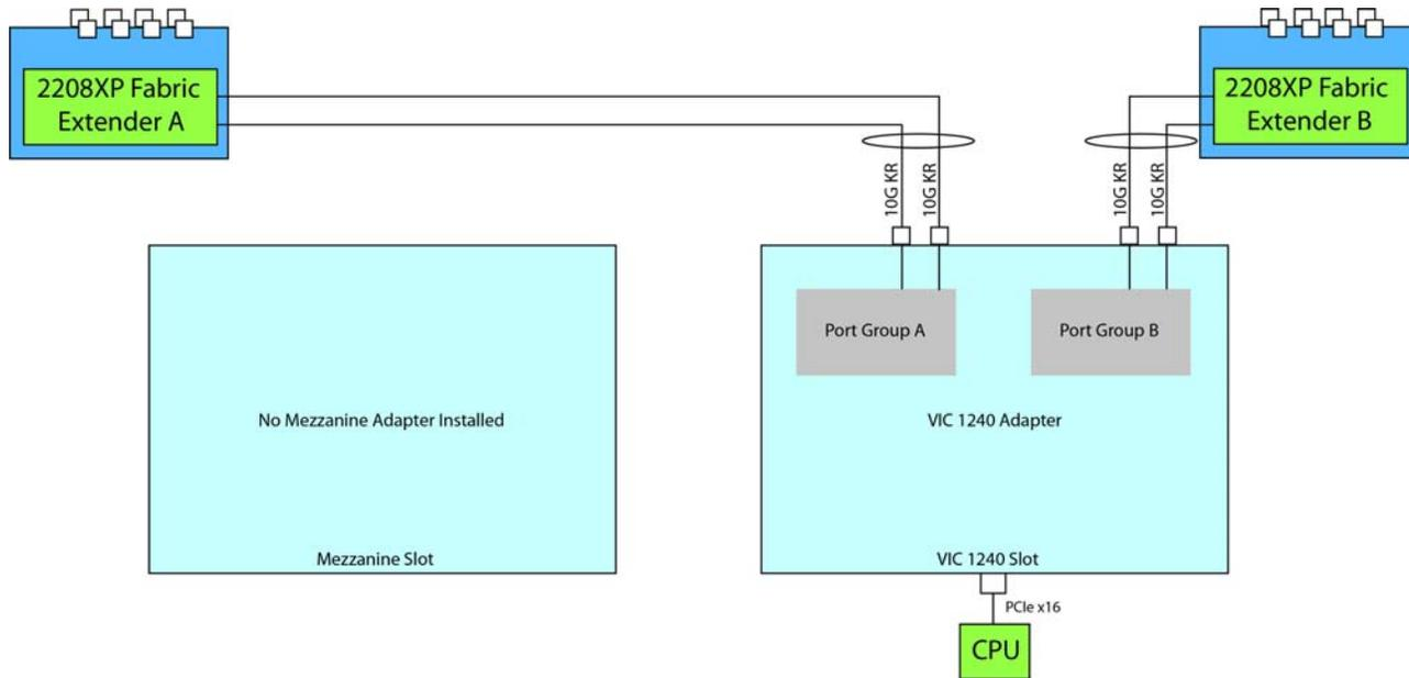
In [Figure 11](#), two ports from the VIC 1240 are channeled to 2208XP Fabric Extender A and two are channeled to 2208XP Fabric Extender B. The Port Expander Card for VIC 1240 installed in the mezzanine slot acts as a pass-through device to channel two ports to each of the Fabric Extenders. The result is 40 Gbps of bandwidth to each Fabric Extender.
