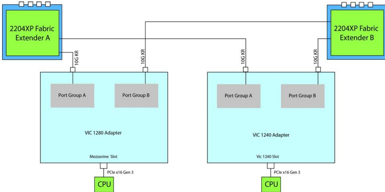
In *Figure 22*, one port from the VIC 1240 is channeled to 2204XP Fabric Extender A and one is channeled to 2204XP Fabric Extender B. The adapter installed in the mezzanine slot also channels one port to each of the Fabric Extenders. The result is 20 Gbps of bandwidth to each Fabric Extender.
