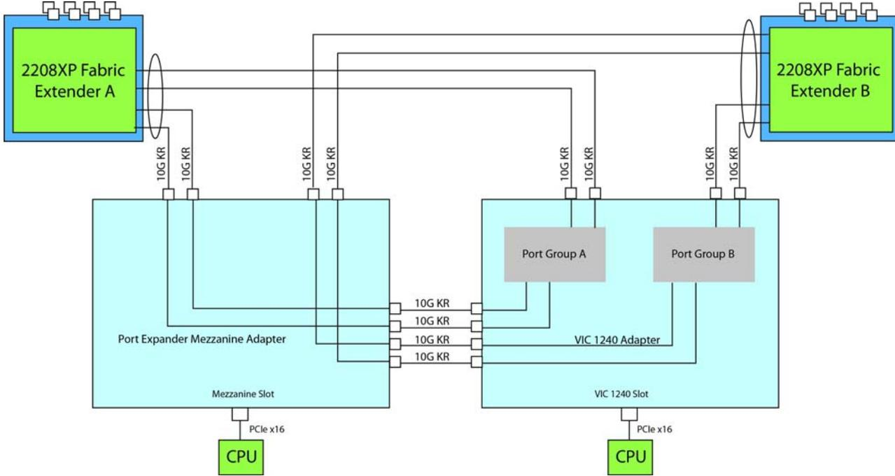
In *Figure 19*, there is no VIC 1240 adapter installed. In this case, a network adapter must be installed in the mezzanine slot. Port A and B of the mezzanine adapter connect to the Fabric Extenders, providing 10 Gbps per port.
