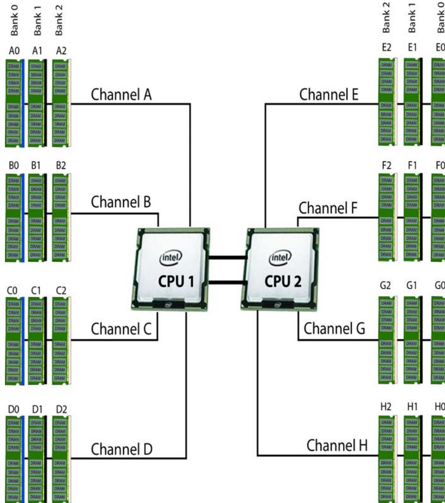
Each CPU controls four memory channels, as follows:
