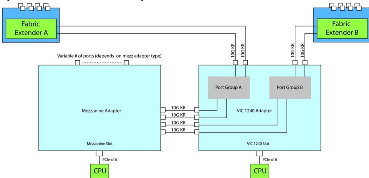
The number of ports available at the mezzanine adapter depends on the type of mezzanine adapter that is plugged into the mezzanine slot on the system board. The maximum number of ports is four. The VIC 1240 senses the type of adapter plugged into the mezzanine slot. In the event a Port Expander Card for VIC 1240 occupies the mezzanine slot, the four 10G KR ports between the adapters are used for port expansion; otherwise, they are unused.
