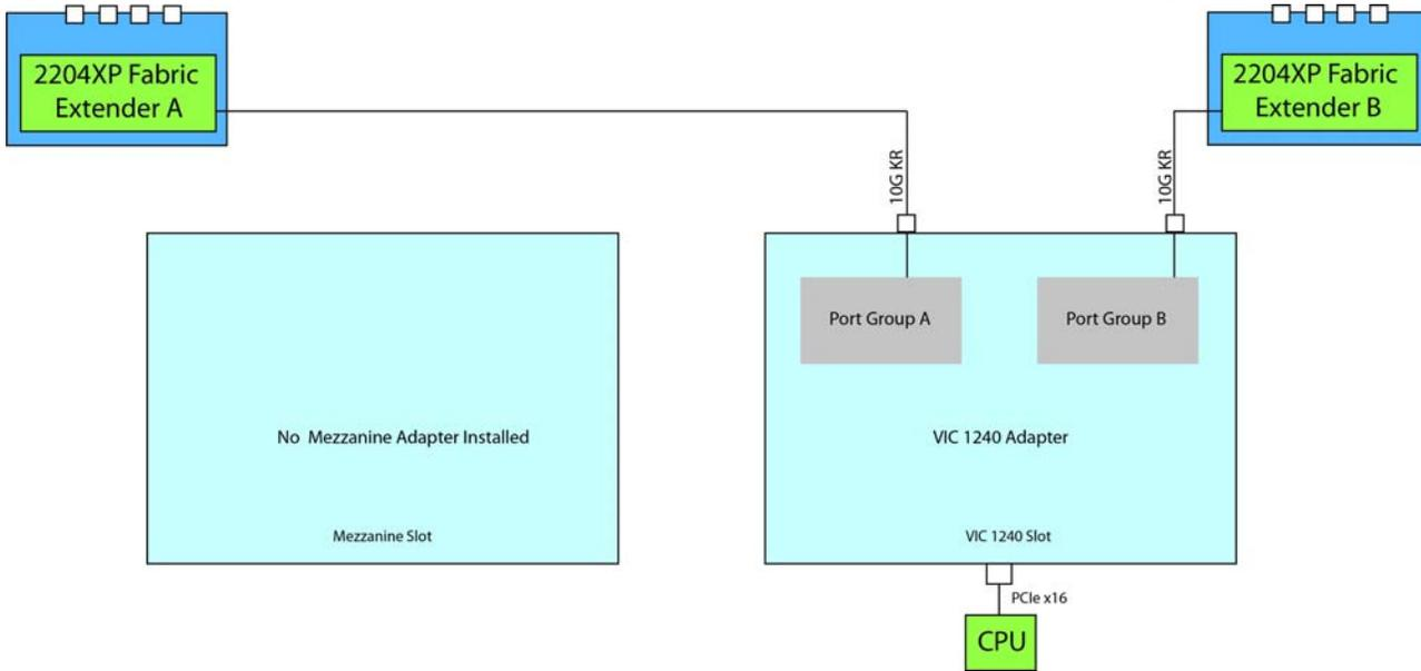
In *Figure 13*, one port from the VIC 1240 is channelled to 2204XP Fabric Extender A and one is channelled to 2204XP Fabric Extender B. The Port Expander Card for VIC 1240 installed in the mezzanine slot acts as a pass-through device to channel one port to each of the Fabric Extenders. The result is 20 Gbps of bandwidth to each Fabric Extender.
