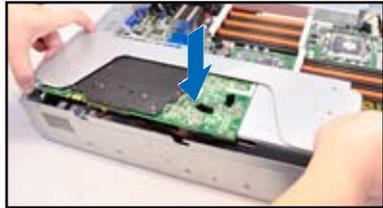
12. Attach the white end of the 8-pin power cable to the 8-pin power connector in front of the GPU computing module bracket.
