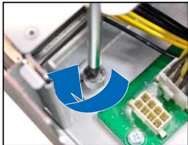
14. Secure the GPU computing module brackets to the server chassis with four screws.
