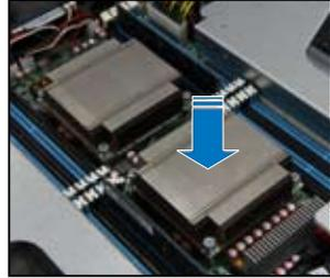
2. Twist each of the four screws with a Philips (cross) screwdriver just enough to attach the heatsink to the motherboard. When the four screws are attached, tighten them one by one to completely secure the heatsink.
