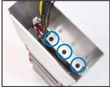
6. Thread the white end of the 8-pin power cable through the GPU computing module bracket.
