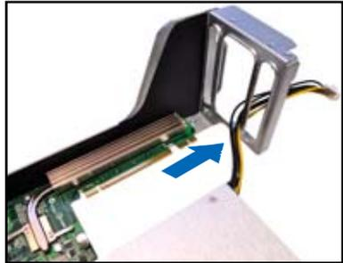
7. Align and insert the golden fingers of the GPU computing module into the card slot on the bracket. Ensure the card is completely seated on the slot.
