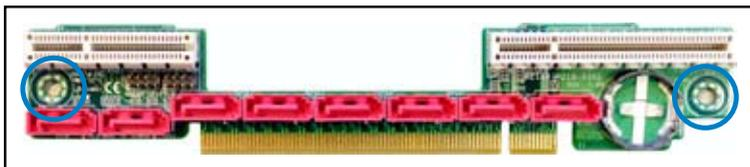
4. If you are to install PIKE 1064E RAID card, secure the riser card to the bracket with two screws. If you are to install PIKE 1078, 2008, 2008/IMR and 2108 cards, secure only one screw, as shown in the right figure.
