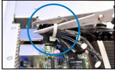
6. Connect the SGPIO cable to the SGPIO1 connector into the SGPIO2 connector on the PIKE riser card.
