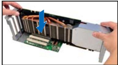
8. Secure the rear end of the GPU computing module to the bracket with two screws.
