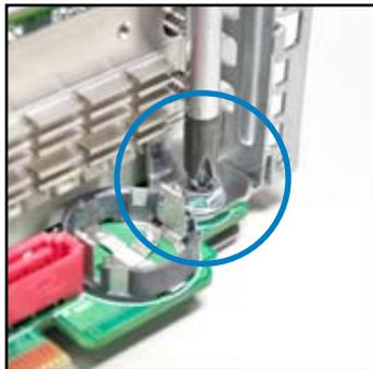
12. For PIKE 1078 SAS RAID card, snap the i Button into the i Button slot on the PIKE raiser card.
