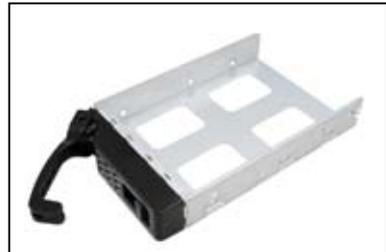
4. Place a SATAII/SAS hard disk drive on the tray, then secure it with four screws.
