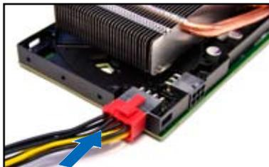
4. Thread the white end of the 8-pin power cable through the airduct of the GPU computing module.
