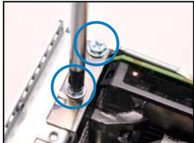
9. Secure the front end of the GPU computing module to the bracket with one screw.
