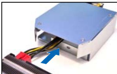
5. From inside the airduct, secure the airduct to the GPU computing module with 3 black screws.
