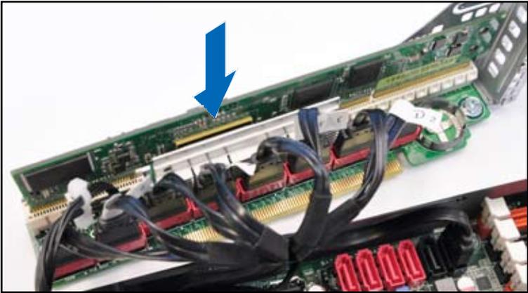
11. If you are to install PIKE 1078, 2008, 2008/IMR and 2108 cards, ensure the heatsink latch is completely hooked to the edge of the card slot, and then secure the PIKE card through the screw hole of the riser card to the card bracket.
