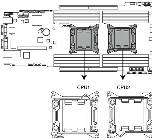
2. Press the left load lever with your thumb (A), then move it to the left (B) until it is released from the retention tab.
