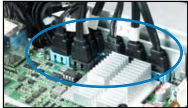
8. The SATA/SAS cables are tied and labeled in four groups. Group 1 connects to HDD 1 and 2, Group 2 to HDD 3 and 4, Group 3 to HDD 5 and 6, and Group 4 to HDD 7 and 8.
