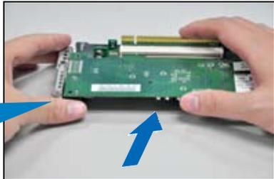
4. Press the riser card bracket until the golden connectors completely fit the slot and the bracket aligns with the rear panel.
