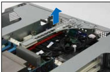
2. Locate the two screws on the riser card bracket, then remove the screws from the bracket.
