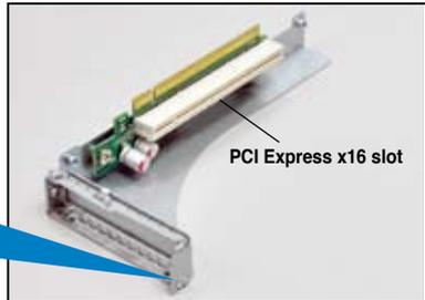
3. Install a PCI Express x16 card to the bracket as shown, and then secure the card with a screw.
