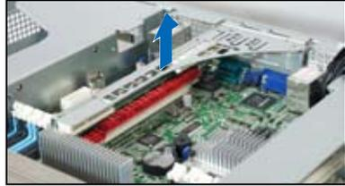
2. Place the riser card bracket on a flat and stable surface, and then remove the screw from the slot bay.
