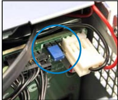
14. Align the riser card bracket to the PCI Express x16 slot on the motherboard.
