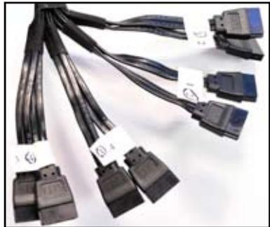
9. Connect the SATA/SAS cables to the SAS1–8 connectors on the PIKE riser card.
