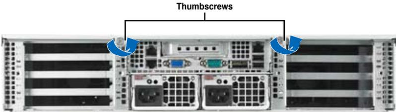
3. Firmly hold the cover and slide it toward the rear panel for about half an inch until it is disengaged from the chassis.
